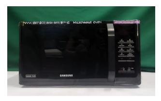
Microwaves are high frequency electromagnetic waves the energy released enable the microbiological media to be heated without changing either the form or the colour. Microwaves generated by the magnetron reflected at cavity and are distributed uniformly as the media rotates on the turntable.
