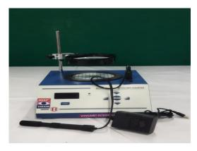
Colony counter is an instrument, used to count microbial colonies on a agar plate containing a growth medium.
