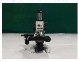
The Light Microscope enables us to view things that are too small to be seen with the naked eye. It uses a system of two or more lenses to collect and focus the transmitted visible light through a specimen to the eye. Animal cells, plant cells, protozoa and bacteria can be easily seen
