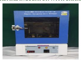
Incubator shaker is a temperature controlled instrument which is carried out both incubation and shaking functions, used in cell culture, fermentation, hybridization under controlled temperature and shaking speed.
