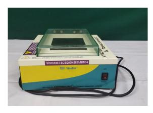
Transilluminator is used to study the results of electrophoretic patterns accurately. Gels after staining are placed on transilluminator and image can be seen directly by naked eye.
