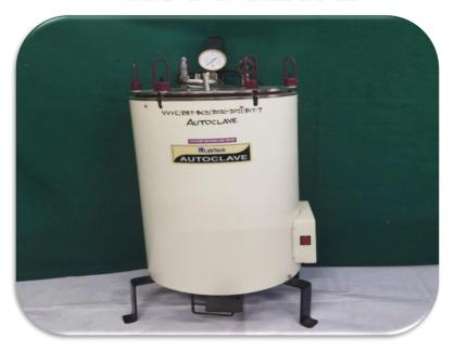
Autoclave is a specialized equipment designed to deliver heat under pressure to a chamber, with the goal of sterilizing the contents of the chamber. The autoclaving process is typically used to destroy microorganisms and disinfect labware, equipment.
