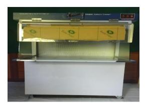
Laminar Air flow chamber is used to transfer the microbial culture in aseptic condition. This equipment is used for providing an excellent aspetic worktable for processes like sub-culturing, inoculation, assays sterile drug preparation etc.,
