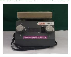
A hot plate magnetic stirrer is used for mixing and heating aqueous solutions simultaneously to speed up the reaction and dissolve the solute in the solvent.
