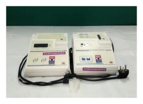
Photo colorimeter measures the intensity of colour concentration of any substance in the solution. The intensity of colour of a substance is in direct proportion to its concentration which in turn is measured in terms of transmittance / optical density.
