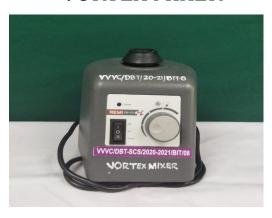
The vortex mixer is a bench top vibrator designed to operate with direct ON and Speed control option. The instrument is designed for vortex mixing of liquids in laboratories, school or factories.
