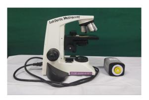
LCD Digital Microscope is an efficient tool to analyse various objects from microfabricted parts to large electronic divices. It can be connected to a TV or Projector for demonstation work. V.V.Vanniaperumal College for Women, Virudhunagar, Tamilnadu No. HRD-11011/163/2020-HRD-DBT/Dt. 24.08.2020/ Biotechnology/SOP for the Equipments
