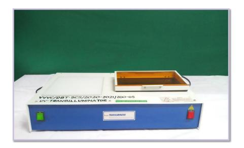
This instrument is used in molecular biology to visualize the proteins, DNA or RNA bands separated using Gel Electrophoresis
