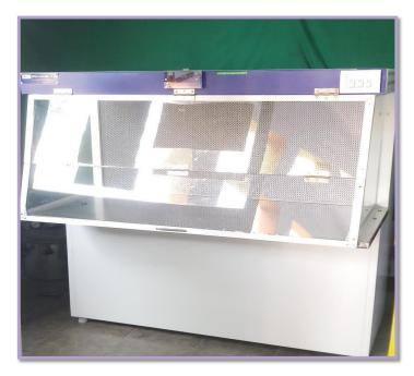
Laminar flow chamber is used provide a filtered airflow across the work area to prevent the airborne contamination in the samples.
