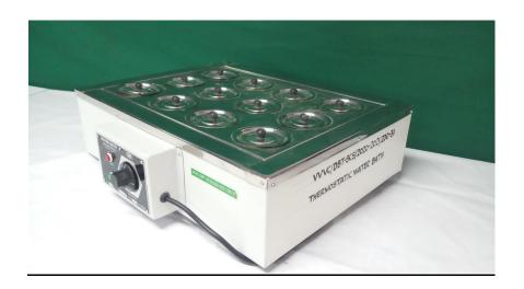
Thermostatic water bath is used for incubation of test samples underwater at constant temperature over a longer period of time.
