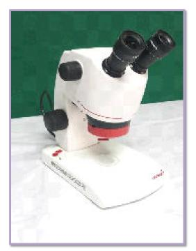
Stereomicroscope is used to examine the opaque specimens and provide 3D view of the insects or any part of the plant that are normally visible to the naked eye.
