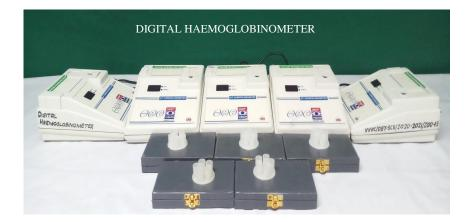
The Digital Hemoglobinometer is a portable device used to measure the concentration of haemoglobin in blood. The measurement of haemoglobin is important to diagnose anaemia or high haemoglobin levels in the assessment of changes before and after operations or blood transfusion.
