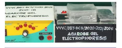
Agarose gel electrophoresis is a general term that is used for the separation of charged particles (ions), the DNA under the influence of an electric field.
