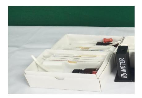
It is an instrument used to determine the quantity of haemoglobin in the blood. It is based on comparision of the colour of the tested blood, which is treated with hydrochloric acid, with the colour of standards V.V.Vanniaperumal College for Women, Virudhunagar, Tamilnadu No HRD-11011/163/2020-HRD-DBT-SCS /2020-2021/Zoology /Standard Operating Procedure/Equipments
