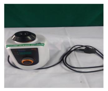
The Vortex Mixer is used to agitate samples and promote homogenization
