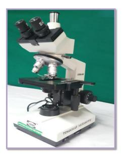
A trinocular microscope is used to take pictures and also record videos of the specimens to be observed. It has two eyepieces like a binocular microscope and an additional third eye tube for connecting a microscope camera V.V.Vanniaperumal College for Women, Virudhunagar, Tamilnadu No HRD-11011/163/2020-HRD-DBT-SCS /2020-2021/Zoology /Standard Operating Procedure/Equipments
