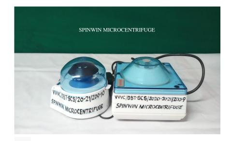
Spinwin micro centrifuge helps to accommodate PCR tubes and micro centrifuges for continuous separations of components in a sample with safety lid lock and lid drop protection.
