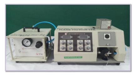
Flame Photometer is used to estimate the concentration of calcium, sodium and potassium in the sample.
